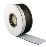
DRG outdoor window connecting film consists of a plasterable non-woven composite laminated on one side or alternately with butyl or self-adhesive. The outdoor connection film is used for quick and safe external, driving rain-proof and diffusion-open sealing of window connection joints and is used as a plasterable external seal.
