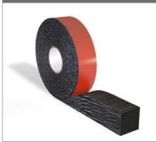
DRG Multiband 3D Premium 900 X is made of a flexible open cell polyurethane foam impregnated with a flame retardant acrylic impregnate. The surface of the tape facing the interior of the building is coated with a thin polymer film. It has a solvent-free, single-sided self-adhesive backing to aid installation. DRG Multiband 3D Premium 900 X is manufactured without halogenated flame retardants, solvent-free, silicone-free, and not using (H)CFC/CHC.
